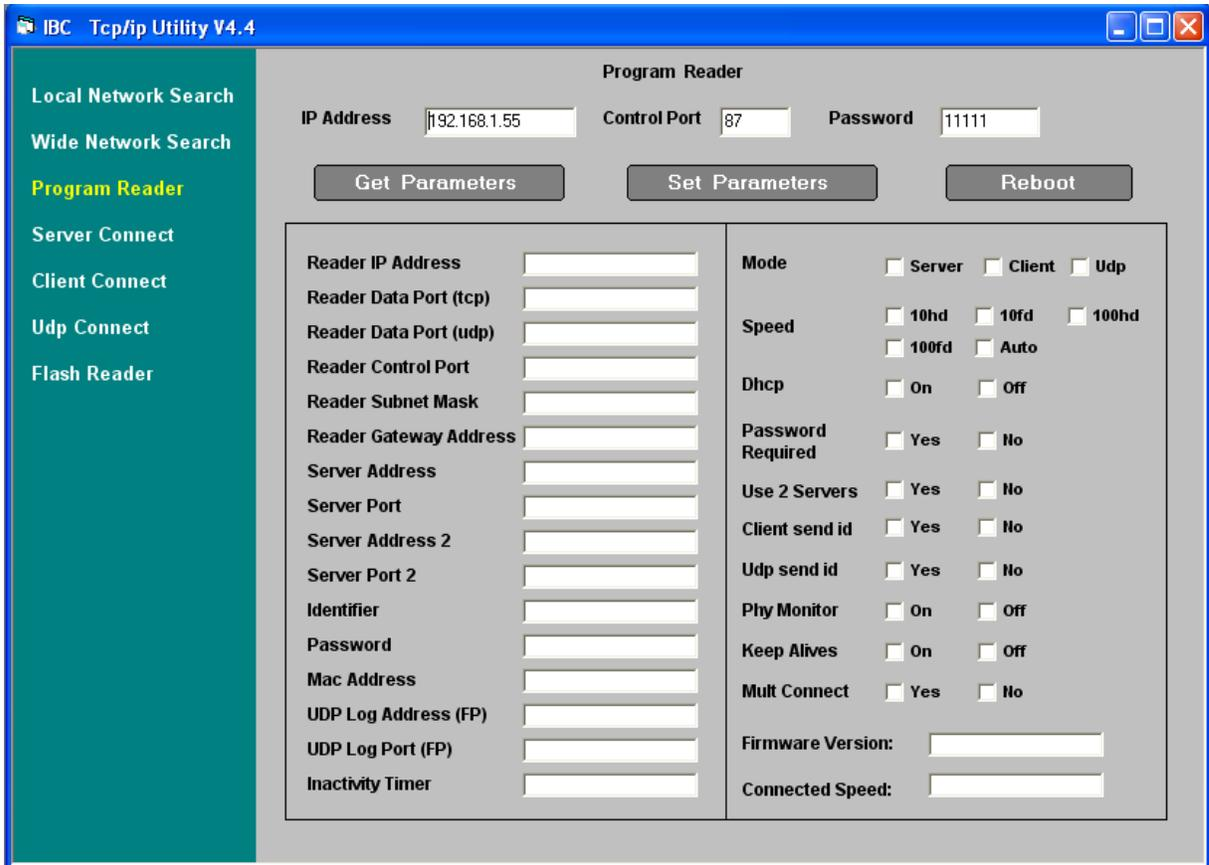
To program a reader, enter in the IP address for the reader and also the Control Port Number. You will also need to enter in the 5-character password. Click *Get Parameters* and the current settings in the reader will be displayed. Note that the password field will be blank and the Mac Address, Firmware, and Connected Speed fields will not be enabled. Two other fields (UDP Log address and UDPO Log port) also will not be enabled. These are for future use.
