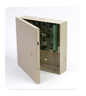
2-Door controller available with Tcp/ip and Rs232. The 8000 is the industry's first controller which can power readers and door strikes directly using POE.
