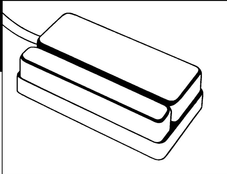
The Magbar-U combines a Barcode Slot Reader and Magstripe Swipe Reader into one device. Output from the Magbar-U is undecoded and may be connected to any standard barcode decoder and magstripe decoder.
