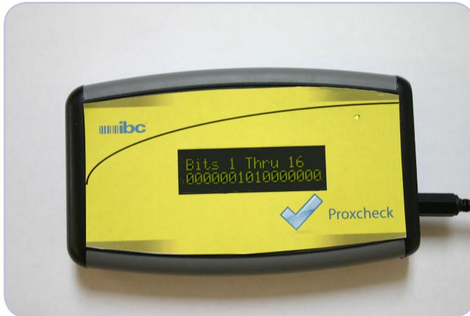
Easily identify and validate your Iclass® cards and fobs with Proxcheck-IC. Proxcheck-IC displays the card data in binary, hexadecimal and numeric formats. The Proxcheck-IC reads cards up to 64 bits in size. Useful for field diagnostics and identifying card numbers for cards with worn-off printing.
