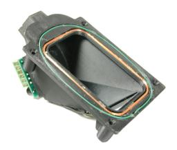
Integration of multiple technologies was never this easy. With Qscant you can read 1D and 2D barcodes, proximity cards, and 13.5mhz smart cards including Iclass SE and Mifare. Qscant is also optimized to read 2D barcodes from cell phones.
