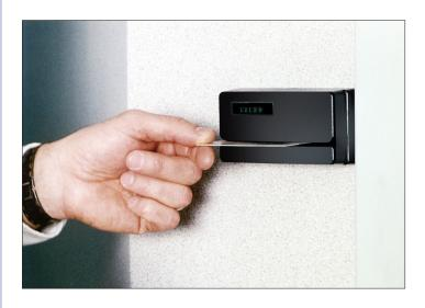
The Smart Prox STAx is a stand alone proximity reader with internal memory, timeclock, and audit trail. The reader contains an internal relay which is used for door control. Access is controlled by validation of badge numbers stored in the internal memory of the reader. Valid numbers can be downloaded into the reader from a PC or scanned into the reader by hand. Optional barcode and magstgripe reading.
